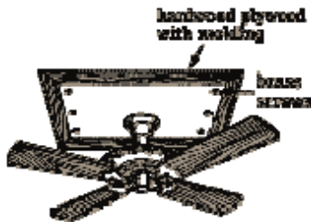
A hardwood plywood panel will cover the large hole in the ceiling made in building a secure mounting system.
